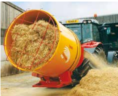
Screens can be changed, with hole diameters from 3/8" - 5"
